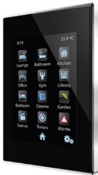
Heating and Cooling Controls within the apartment is achieved by the Zennio Z41PRO control panel. This will activate automatically (or manually if required) the system needed to reach the temperature desired.
