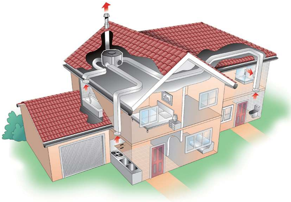
Figure 1.1C - An MEV Schematic Diagram
