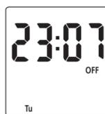
WHERE THE DAY AND TIME ARE CORRECT, BUT THE ON/OFF INDICATOR MAY NOT REFLECT THE CURRENT PROGRAMME ACCURATELY, IN WHICH CASE PRESS THE ADV BUTTON TO CORRECT THE INDICATOR.
