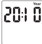
PRESS TIME REPEATEDLY UNTIL THE MINUTES ARE SHOWN. USE ADV OR BOOST TO CHANGE THE MINUTES TO THE CORRECT VALUE. PRESS TIME TO RETURN TO OPERATING MODE. OTHER CHANGES CAN BE MADE THE SAME WAY, BUT THE TIME BUTTON MUST BE PRESSED TO RETURN TO OPERATING MODE AFTER ANY CHANGES, THERE IS NO AUTOMATIC EXIT FROM TIME/DATE ENTRY MODE.
